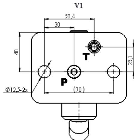
3-way selector valve for Massey Ferguson, to be installed directly on the lift cover
