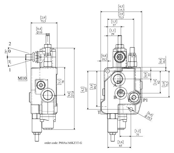
Applicable in both horizontal and vertical log splitting machines. It is characterised by the function of rapid approach to the log with maximum flow and pressure <70 bar and when the log is reached automatic switch to low flow rate and maximum pressure.
